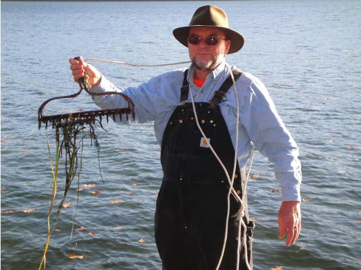
Figure 6. Aquatic plant sampling rake comprised of the heads of two garden rakes wired together (13” long) and tied to 33’ of woven nylon line (5/16 inch diameter; clothesline).
