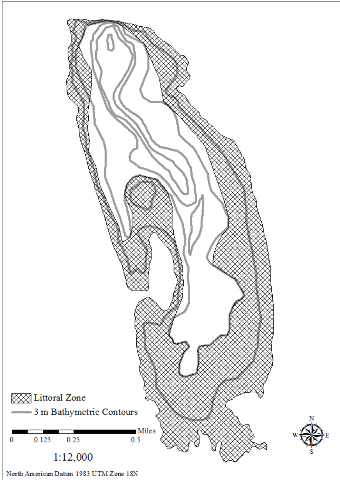
Figure 5-2. Estimated littoral zone of DeRuyter Reservoir based on surveys conducted during the 2016 growing season and bathymetric mapping.
